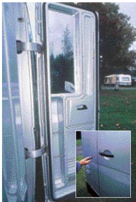
Like the rest of the body, the caravan door is of good quality. Clever hinges let it open wide and close flush. Inset: The caravan door lock is operated by the base vehicle ignition key.
