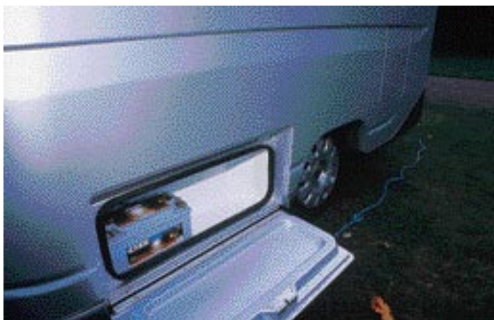
The leisure battery locker has room for a second unit if needed.
