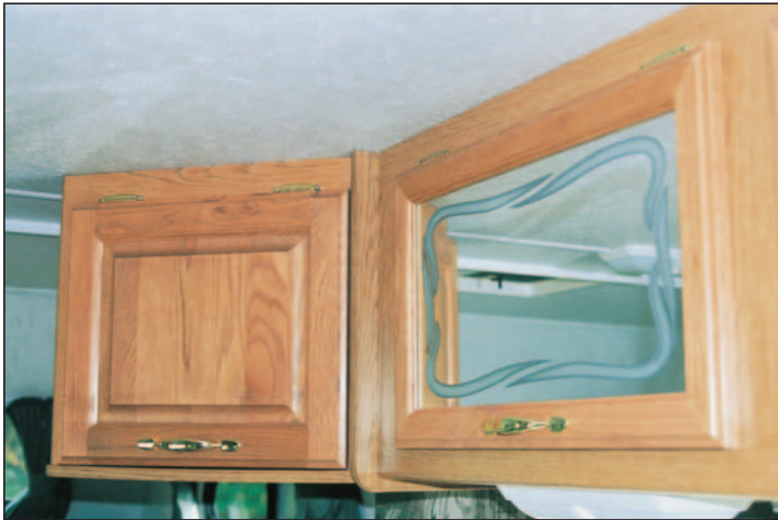
All locker doors are in raised oak, or have etched glass mirror inserts. The latter are a typical feature of American RVs.
