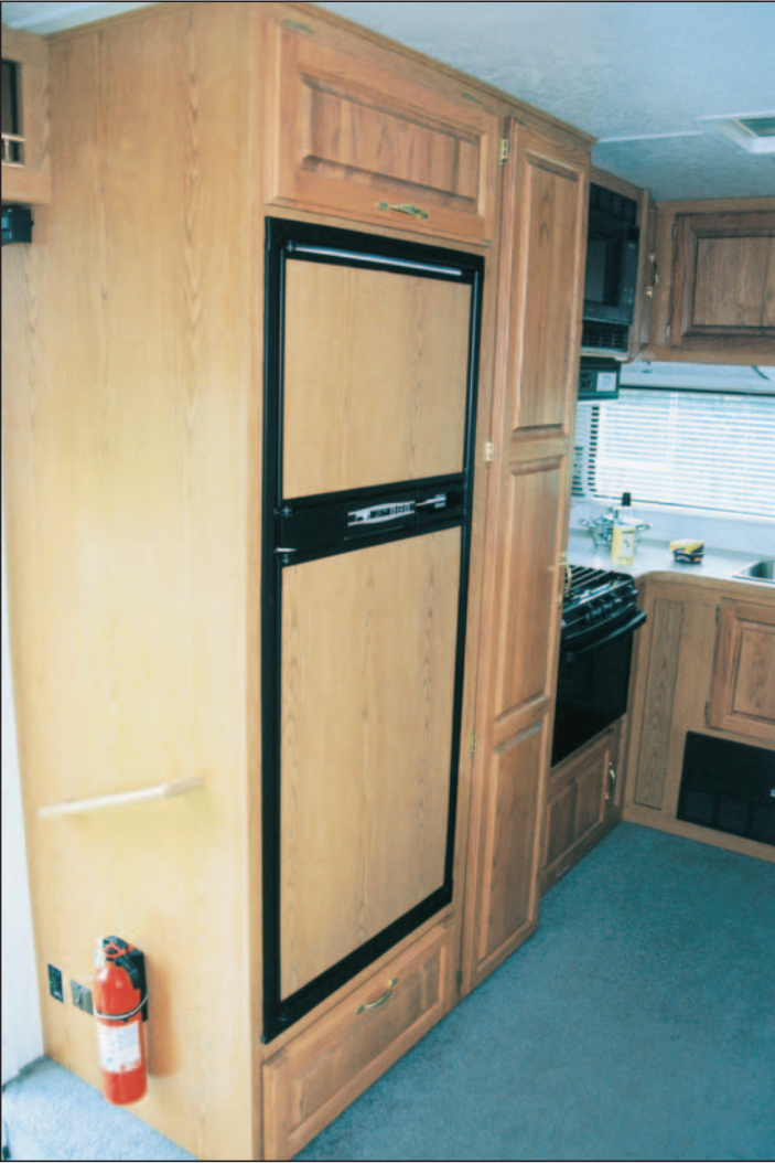
Gigantic three-way Norcold fridge/freezer is adjacent to the entrance door. Moving towards the rear there is a full-height larder followed by...
