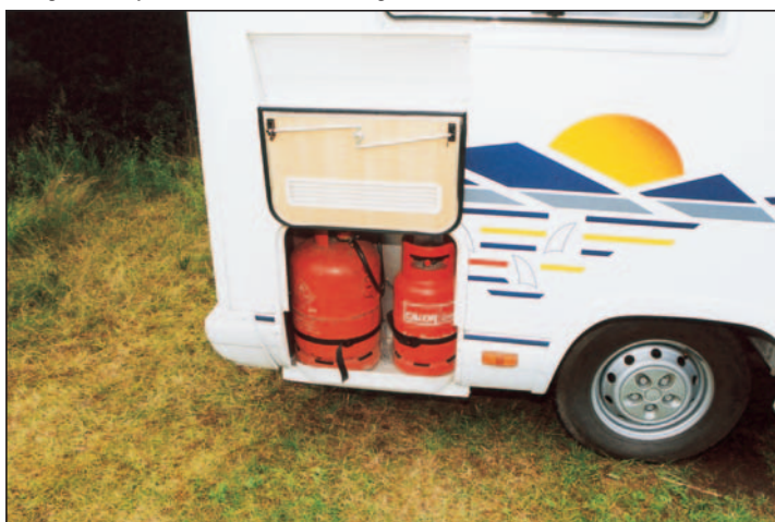
Rear offside corner is home to the gas locker, which will hold two 13kg cylinders - more than most rivals.
