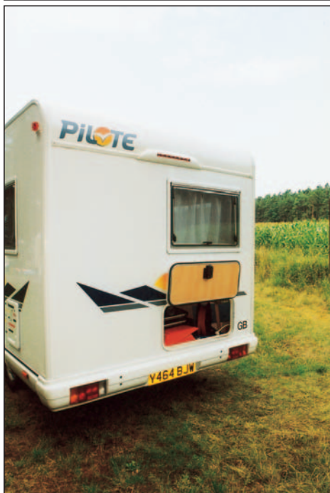
Unusually this Pilote has its access to the underbed locker at the rear, rather than the side. Hatch is big enough to accept outdoor chairs or a folding bike.
