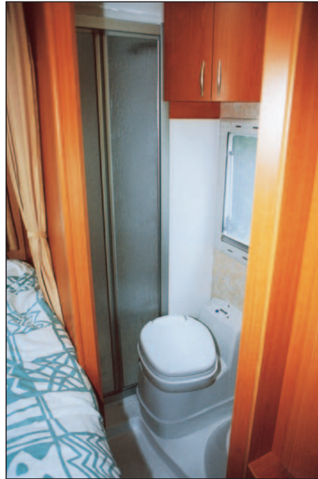
Beyond the toilet is the separate shower with proper folding doors. There's plenty of room to shower and a large bore drain hole ensures that water flows away well.
