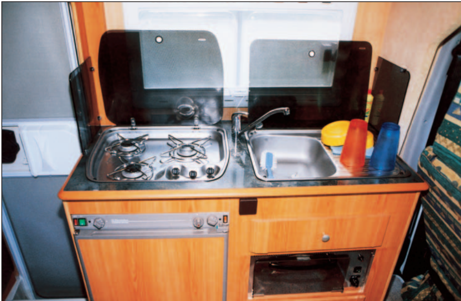
The kitchen again - opened for action. Hob has three burners, but no spark ignition. Stainless steel sink has integral drainer.
