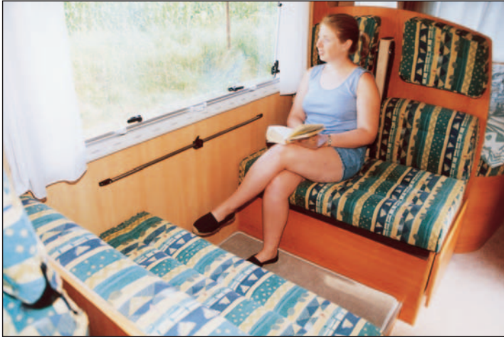
Forward-facing dinette seat has head restraints and three-point belts, but upright seatbelt mounting could be better hidden and protected. False floor between seats ensures comfortable seat height.
