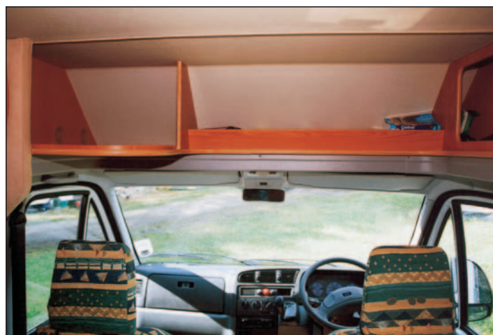
The cab roof has been cut away for an easy walk through. On the left is a TV shelf (but no power point) and a shelf above the 'screen is perfect for guidebooks and maps.
