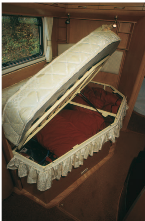
Access to the locker under the fixed bed is easy, with gas-strut assistance.
