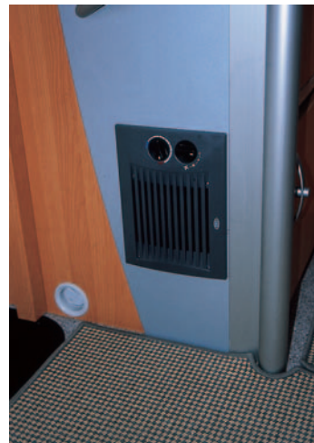
The optional heat exchanger uses waste engine heat to warm the body of the 'van when travelling.
