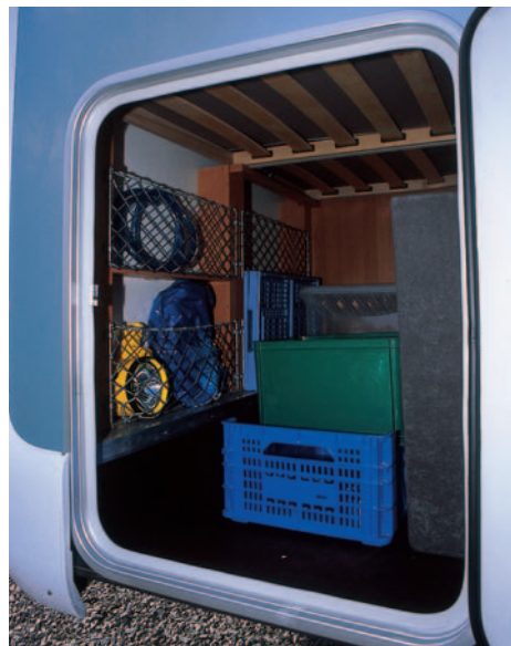
Shelving in the underbed storage locker is usefully kitted-out with stretchy cargo netting.
