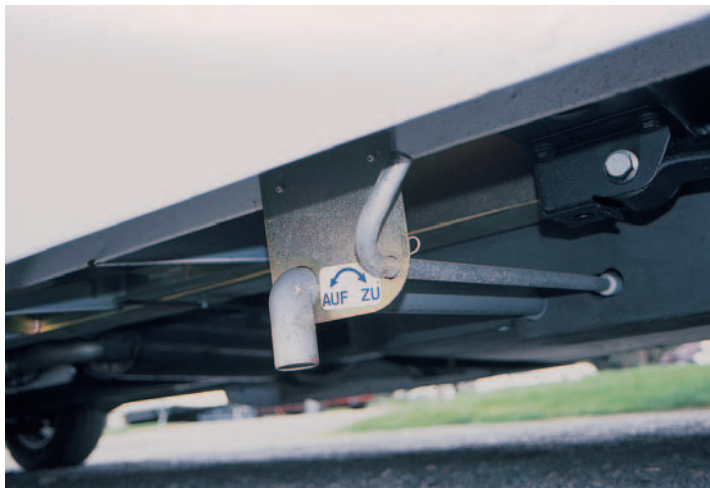
A nice positive anticlockwise turn of a strong metal handle empties the waste water
