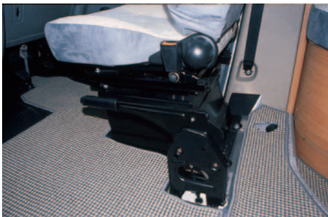
The clever handbrake folds down out of the way after you apply it, allowing the driver's seat to swivel easily.
