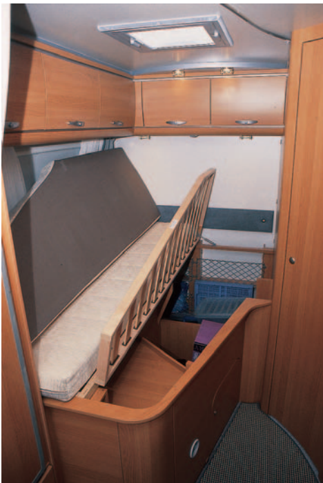
Lifting the hinged slatted mattress support lets you access the big storage area that the higher-than-usual bed creates.
