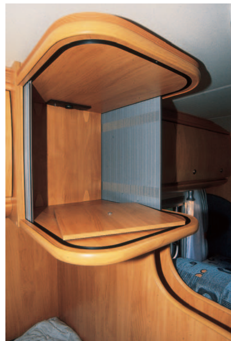
The TV locker features a plinth and its tambour walls retract fully for a good view from lounge or bed.
