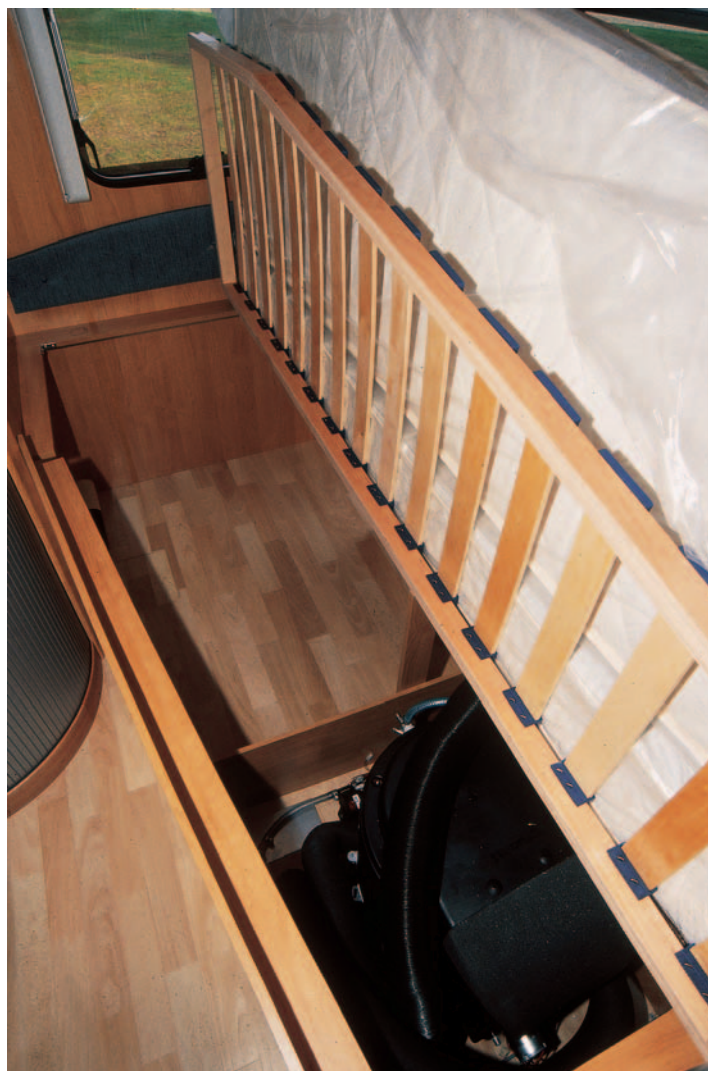
The underbed locker provides a usefully large storage area, as well as a home for the Truma Combi boiler.
