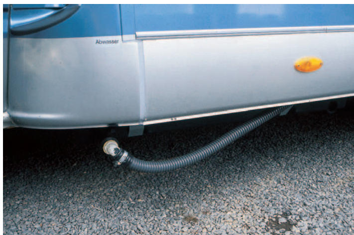
The abwasser drain - and the waste water tank - are vulnerably low.
