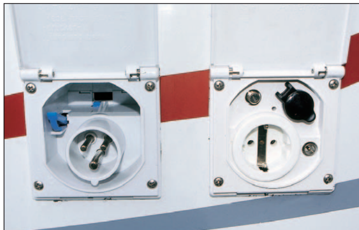
External sockets are for 12V & 230V power 'out and in' and satellite TV.
