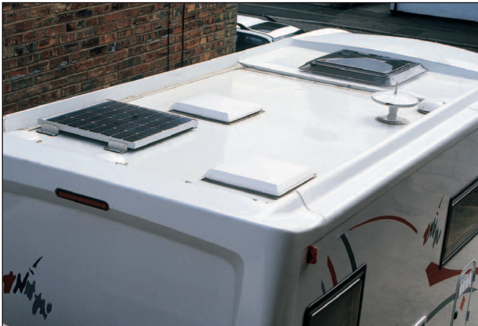
The roof tended to hold water. Solar panel, TV aerial and large rooflight are all standard.
