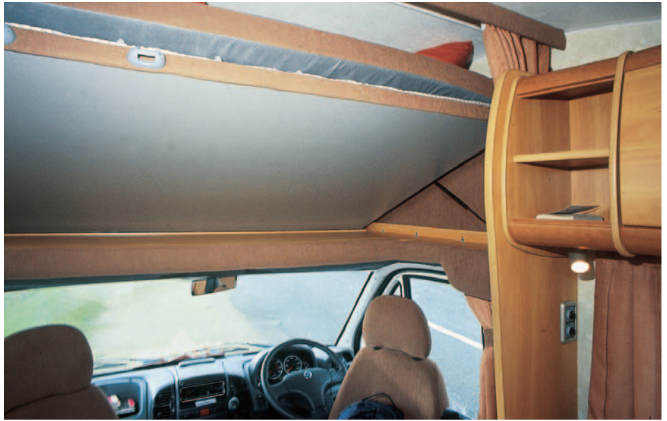
The upper bed lifts into the luton roof with the aid of two gas struts.
