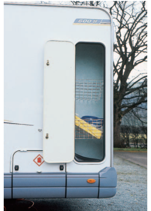
The exterior wet locker. As a ski locker it is fine, but with only outside access the top two feet are inaccessible.
