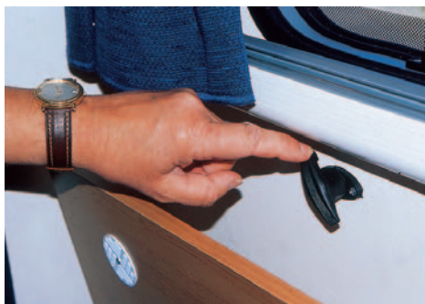
Turnbuckles restrain boards, which hinge down to fill the spaces left by each sliding settee base. The squabs and backrests make a flat mattress...
