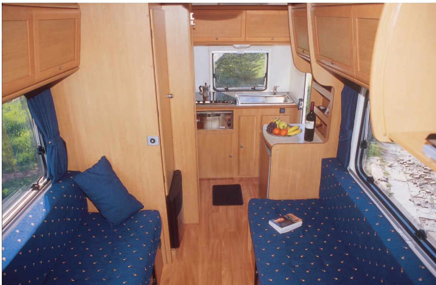
Classic internal layout of front lounge and end kitchen with offside corner washroom.
