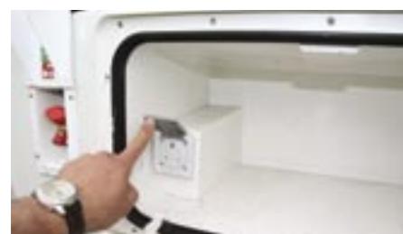
An outside locker socket is a praiseworthy point but would have been neater mounted in the locker wall
