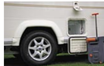
A wheeled toilet with easy-access hatch
