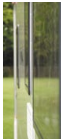
Windows are flush with the bodywork
